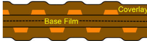
Figure 4.8 Staggered adjacent-layer traces are preferred
