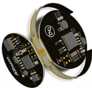
Figure 3.2 Bending up the mechanical model to show design intent
