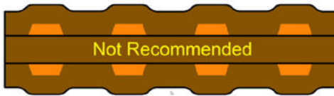
Figure 4.7 Adjacent-layer copper traces are not recommended
